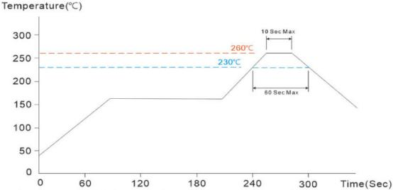
No mechanical and electrical defects are found after testing based on the above profile and keeping under the conditions of room temperature and humidity for 2 hours. Twice reflow test is acceptable with the test interval remaining 1 hour under the normal conditions.
