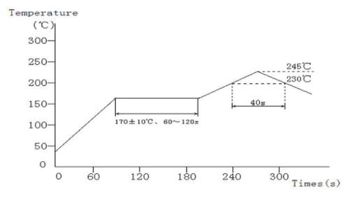
The recommended reflow profile is based on the testing instruments used. Solder ability will depend on the testing equipments, reflow conditions, testing method, etc. So it is necessary to make a confirmation of them when the reflow conditions are set up.
