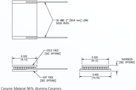
Ceramic Material 96% Alumina Ceramic Solder Construction: 138°C BiSn
