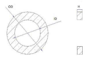
The waterproof and dustproof sound-permeable membrane is treated with nano-hydrophobic and oleophobic surface. Consists of waterproof and dustproof sound-permeable membrane raw material + 3M waterproof stamina glue + PET (Release paper), processed and shaped.
